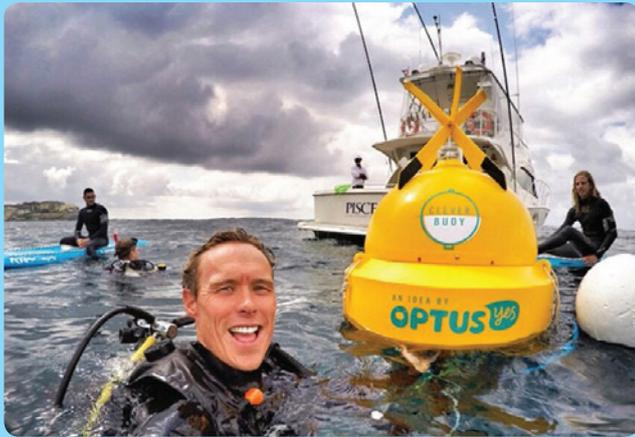
The Clever Buoy uses newly developed sonar interrogation software which detects sharks and transfers a warning system via mobile and satellite communications back to shore. The alert is sent to lifeguards, beach goers and researchers.
